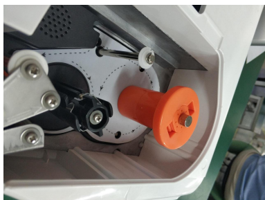
a. Open the dust cover and remove the paper stop block.
